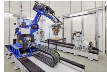
automatic fiber placement (AFP) process
